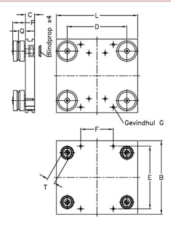
B = 150 C = 18.00 d = 130 E = 130 F = 80 For bearing = 34 For slide = M/NM 76 L = 170 P = 21.3Q = 11.50Threaded hole G =  $4 \times M8$
